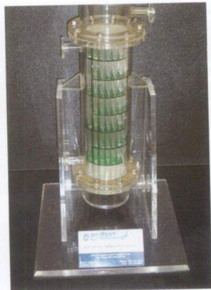
6025 VERTICAL THERMOSYPHON REBOILER
