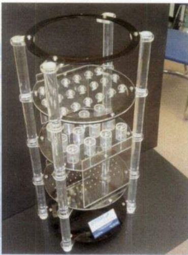
TRAY-2 ACRYLIC DISTILLATION TRAINING TRAYS
