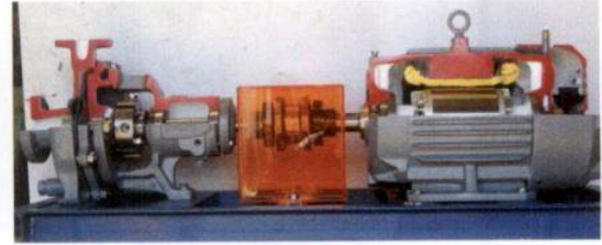
9017 CENTRIFUGAL PUMP SKID
