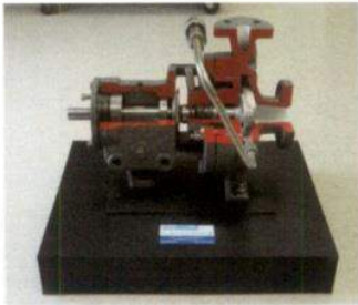
9001 CENTRIFUGAL SINGLE STAGE W/MECHANICAL SEAL
